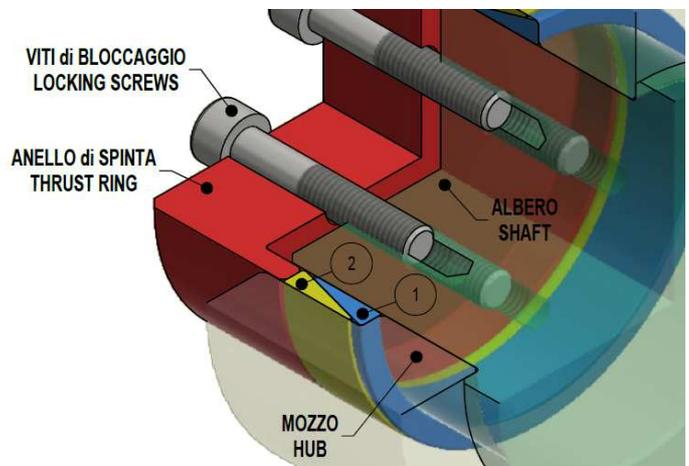
Fig. 3. Design example w/ tapped shaft.
