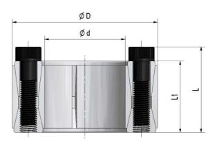
Ma: screw tightening torque Mt: transmissible torque (Fax=0) Fax: transmissible axial load (Mt=0)
