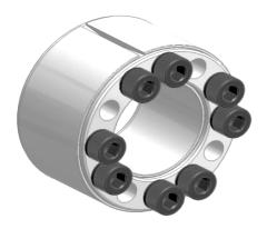
Medium-high torque capacity Self-locking & self-centering Axial fixation of hub during tightening: yes Max tolerances: shaft h9; hub bore H9 Shaft / hub bore surface finish:  $0.8 \le Ra \le 3.2 \ \mu m$
