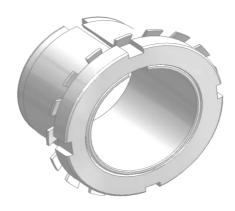
Low torque capacity Low contact pressures Self-locking & self-centering Axial fixation of hub during tightening: no Max tolerances: shaft h8; hub bore H8 Shaft / hub bore surface finish:  $0.8 \le Ra \le 3.2 \ \mu m$
